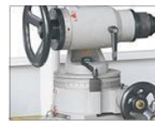
High precision scale ring and control hand wheel
